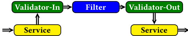
Figure 1. Architecture of a typical application-level network filter. The system pipes all incoming packets through a filter, validating that the packet is well-formed before and after.
